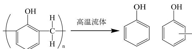
Fig.1 Proposed decomposition reaction path of phenol resin.
