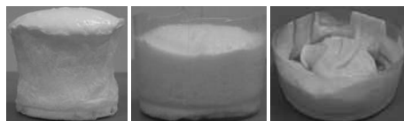
Figure 3. Foaming assays with partial replacement of the commercial polyol by recovered polyol 33% (centre) and 50% (right)
