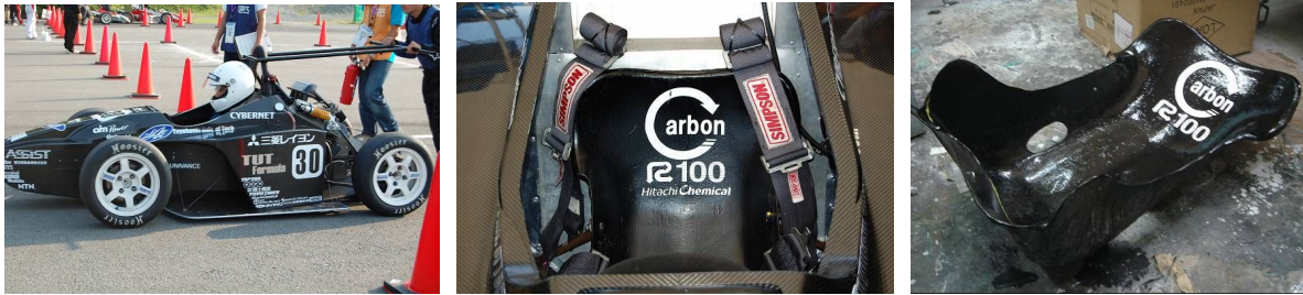
Fig. 6 A driver's seat on the formula car used nonwoven fabric made from recovered CF
