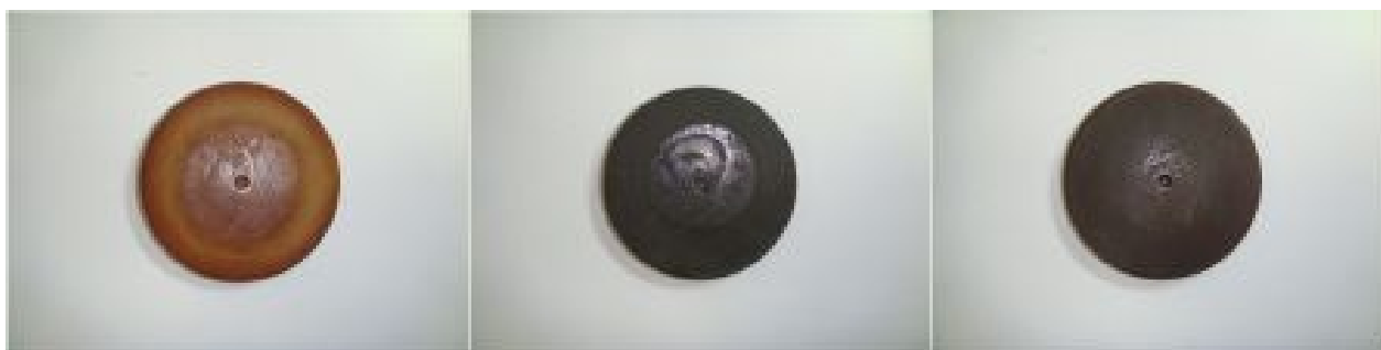
Fig. 1 Obtained polymers from the monomeric material recovered from the reaction in the presence of 1% of DMAP. From left, 20%, 40%, and 60% of recovered monomer was used
