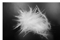
Fig.1. Glass fiber extracted from FRP waste
